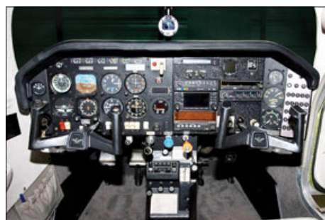
The M20J's front office has more than enough room for everything. Note the engine power gauges on the far right, along with circuit breakers. Fuel and system gauges are top and center, along with the trademark gear switch.
